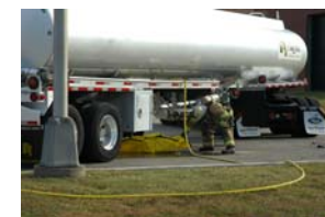
Deploying a containment pit.
